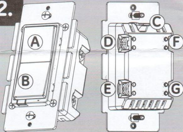
**A. Top Rocker** — (Press & release to turn fan control on, press & hold increases speed)
