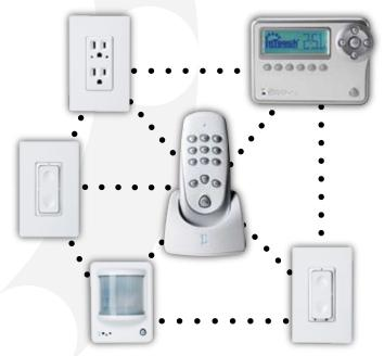
The server also tracks the status of every InTouch device in the network as well as any legacy Z-wave devices. The user is able to instantly see the status of any scene just by looking at control devices like the hand-held remote, multi-scene or master control.
