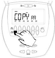
Fig 16d – Press and release the Channel 1 OFF/DIM button on the Secondary Controller . “RA” which stands for “Receive ALL data” will be shown next to “Copy”.
