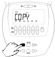
Fig 16c – Press and hold the INCLUDE button on the Secondary Controller . “Copy” will be shown in the LCD display. Release the INCLUDE button.
