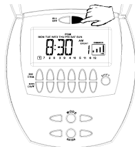
Fig 14f – Press and release ALL ON to use SCENES (preset light levels)
