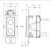
The CA3000 Wall Switch is a Z-Wave™ enabled device which is fully compatible with any Z-wave enabled network. Z-Wave enabled devices display the Z-Wave logo and guarantee connectivity and interoperability between devices. Each line powered node in a Z-Wave network is designed to act as a repeater forming a mesh network eliminating radio "dead spots" and providing the highest level of reliability.
