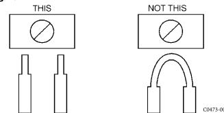
DO NOT loop the wire under the clamping plate.
