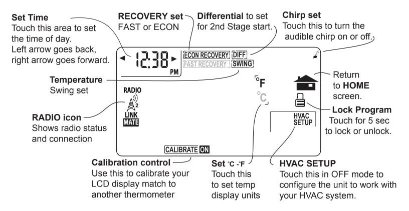
**MANUAL Screen** The **Manual Screen** control screen is where you can make temporary changes to your CT100's operation. From the HOME screen, touch the main temperature display to use this screen. [See page 13 for details]
