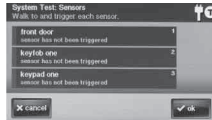
Figure 68. Sensor Test Screen in Walk Test Before Testing
